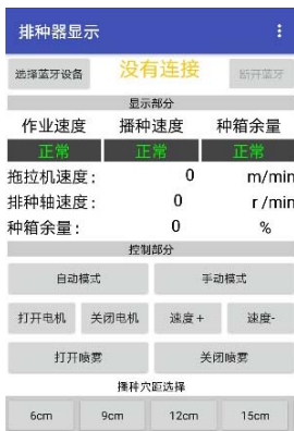
图8 Android终端人机交互界面 Figure 8 Interactive interface of Android mobile phone terminal
