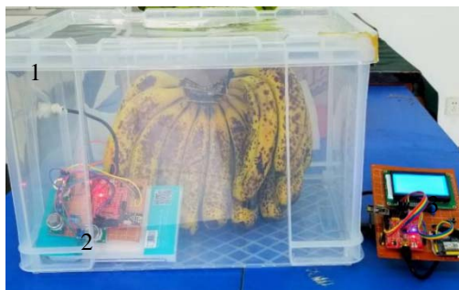
1. 模拟香蕉仓储箱; 2. 数据采集终端; 3. 手持中继节点 1. Simulated banana storage box; 2. Data acquisition terminal; 3. Handheld relay node
