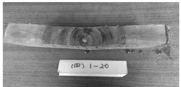
图 1 氯锌碘对杨木横断面染色情况 Figure 1 Surface staining of Poplar with ZnCl_2-I_2
